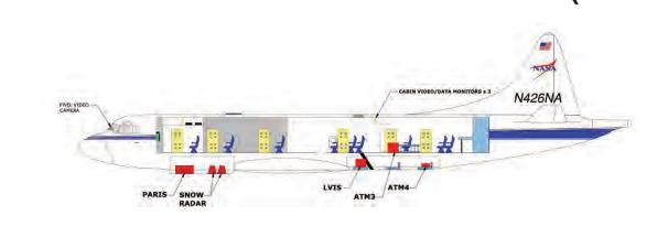
LVIS: Laser Vegetation Imaging Sensor ATM: Airborne Topographic Mapper PARIS: Pathfinder Airborne Radar Ice Sounder Kansas Snow Radar: Sea ice snow depth radar
